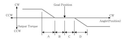
A: CCW Compliance Slope(Address0x1D) = 0x40(Approximately 18.8°)
